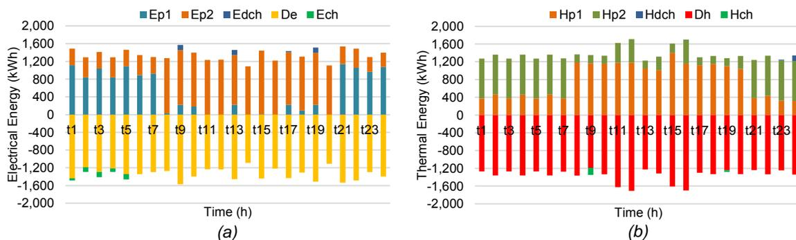
Figure 3: The hourly energy production schedule to satisfy (a) the electrical and (b) thermal loads using OCM.
