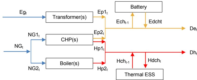
Figure 1: Superstructure of OCM showing the optimal EH design with CHP implementation to consider the integration of transformer(s), CHP(s), auxiliary boiler(s), electrical ESS, and thermal ESS.
