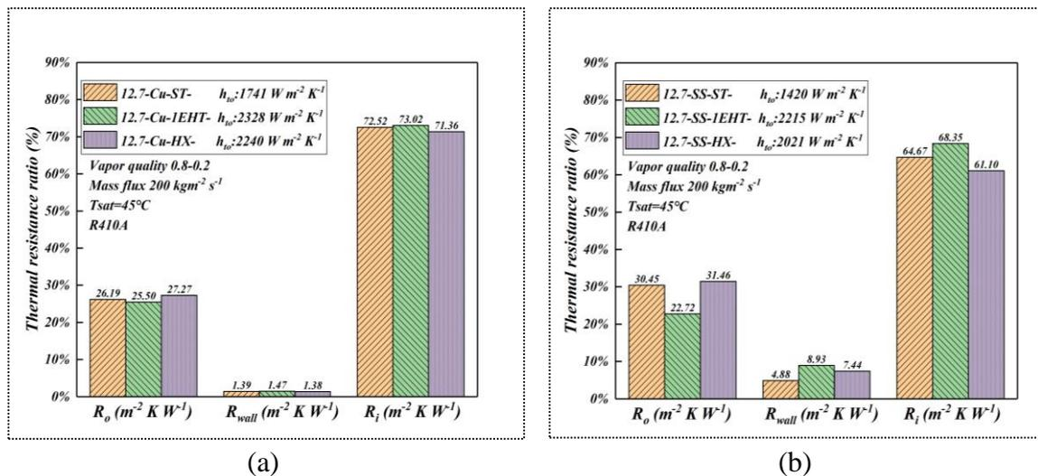
Figure 4: Comparison of the thermal resistance for (a) copper tubes and (b) stainless steel tubes
