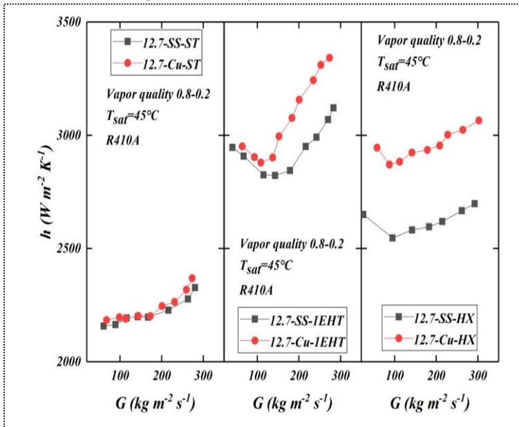
Figure 3: Comparison of condensation heat transfer coefficients inside 12.7-mm-OD copper and stainless steel tubes with various mass fluxes
