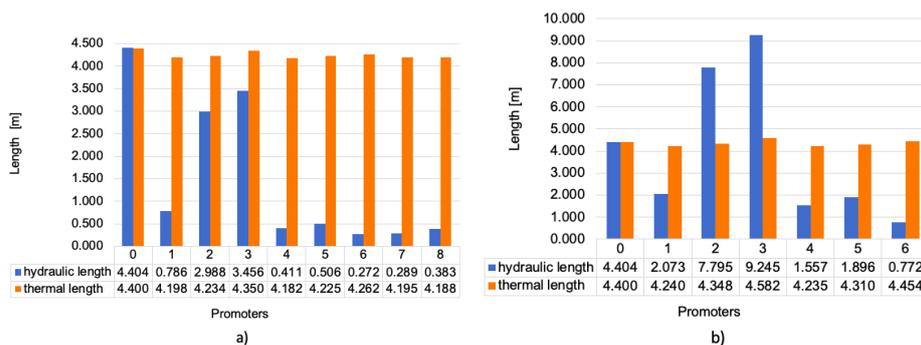
Figure 3: Heat exchanger retrofit considering a viscous fluid: a) Inserts without changing exchanger internals, b) Reduction of number of passes from 4 to 2
