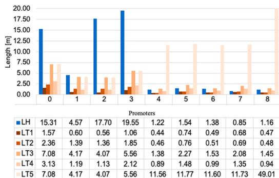
Figure 1: Thermal and hydraulic length considering the effect of opposing stream on the selection of the turbulence promoter
