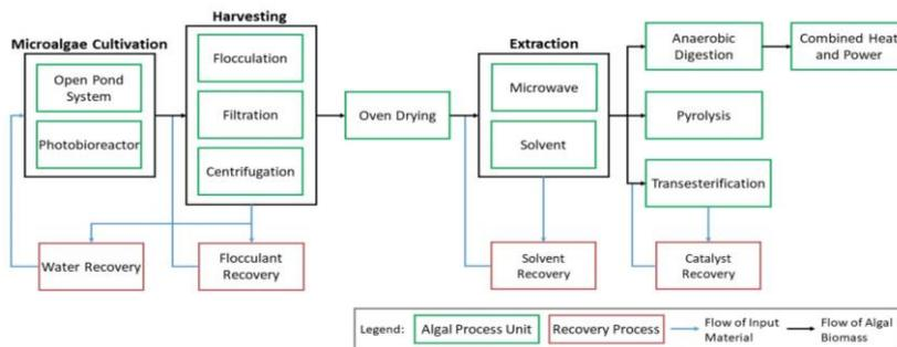
Figure 1: Microalgal biorefinery process network
