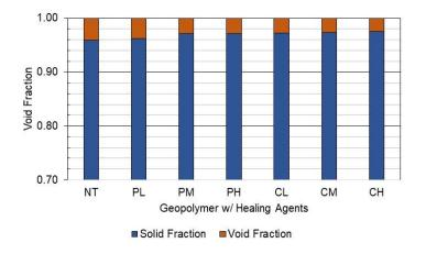
Figure 6: Solid and void fractions of the geopolymers based on image analysis
