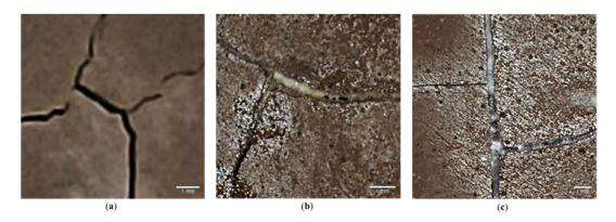
Figure 4: Crack sealing in a geopolymer after 28 healing days—(a) no healing agent; (b) using a pure culture of B. sphaericus, and (c) using co-culture of B. sphaericus and B. thuringiensis
