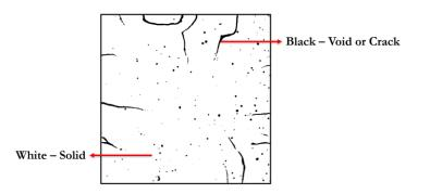
Figure 3: Binary image of a slice of a geopolymer cube
