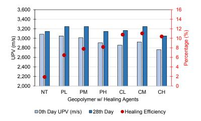
Figure 5: Initial and final UPV and healing efficiency of the geopolymers
