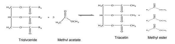
Figure 2: Scheme for stepwise interesterification reaction
