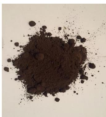
Figure 1: Appearance of ilmenite concentrate ore-thermal melting dust
