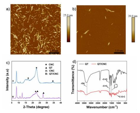
Figure 1: AFM height images of the (a) CNC and (b) QT/CNC; X-ray diffractograms of CNC and QT/CNC (c); FTIR spectra of QT and QT/CNC (d).
