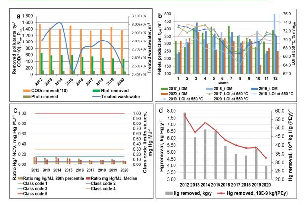
Figure 2: Dynamics of WWTPL: a) outflow, COD, nitrogen and phosphorus removal rate per year, b) pellet's production and LOI at 550 °C, c) SRF classification (ratio Hg/NCV of 10 monthly subsamples), and d) annual removal rate of Hg
