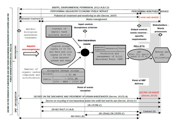
Figure 1: The management system for municipal wastewater treatment and SRF production at WWTPL
