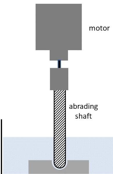
*Figure 1: Simplified scheme of the experimental setup for nanoparticles synthesis.*
