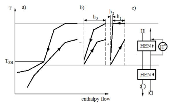
Figure 3: HEN retrofit concept to enable condensate subcooling in selected heaters denoted  $H^*$ : a) Balanced Composite Curves, b) temperature profiles of the heat exchange in heaters  $H^*$  [heat duty h1 and h2], and network part HEN $\uparrow$  [heat duty h3], c) simplified block scheme of the HEN including its parts operated above and below Pinch temperature [HEN $\uparrow$  and HEN $\downarrow$ ]; C – coolers
