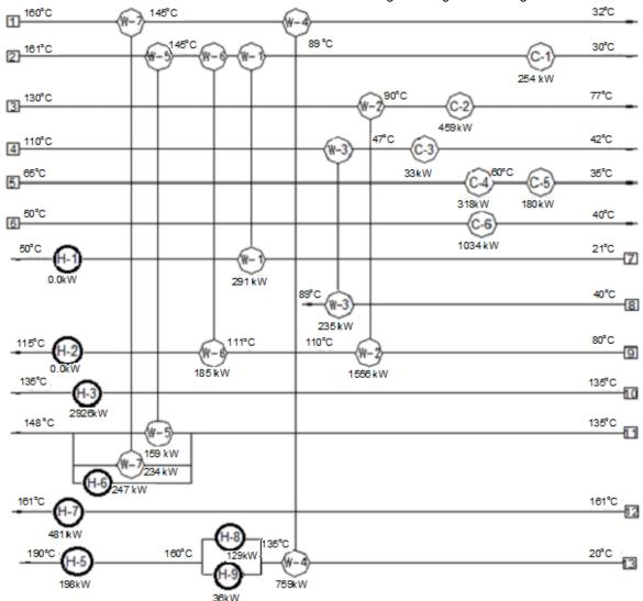
by thermal interactions between hot streams  $(1 \div 6)$  and cold streams  $(7 \div 13)$  in the existing heat exchangers W-1 ÷ W-5 and new ones W-6 and W-7. The waste heat is discharged through the existing coolers C-1 ÷ C-6.
