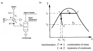
Figure 1: Heat supply from CHP plant to crude-oil heating: a) flow diagram; b) changes in the thermodynamic state of steam and its condensate in the T-s diagram
