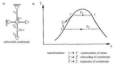
Figure 2: Crude oil heating with subcooling of steam condensate: a) flow diagram, b) changes in the thermodynamic state of steam and its condensate in the T-s diagram
