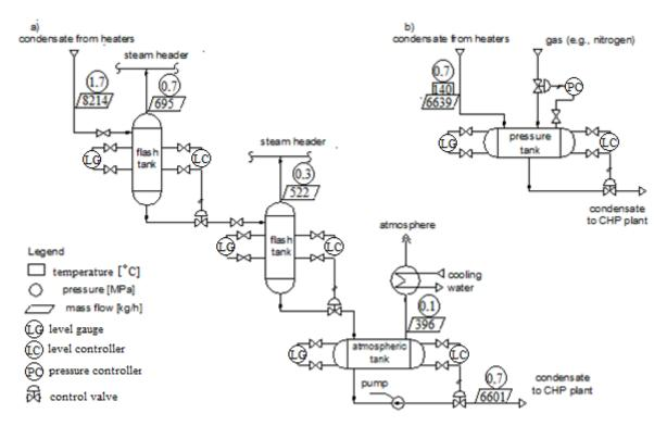
Figure 5: Scheme of condensate management in the MTBE plant: a) condensate flashing in the existing HEN arrangement, b) condensate tank connected to the retrofitted HEN
