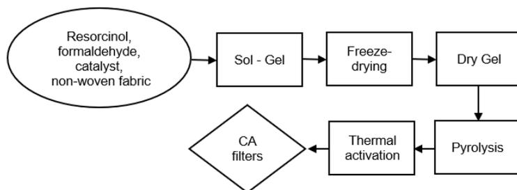
Figure 1: The process of synthesizing carbon aerogel filters
