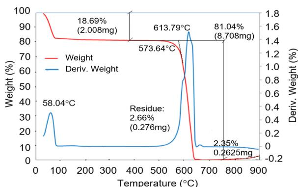
Figure 3: Thermogravimetric analysis (TGA) results for CAF
