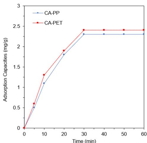
Figure 7: Adsorption capacity of CA-PP and CA-PET
