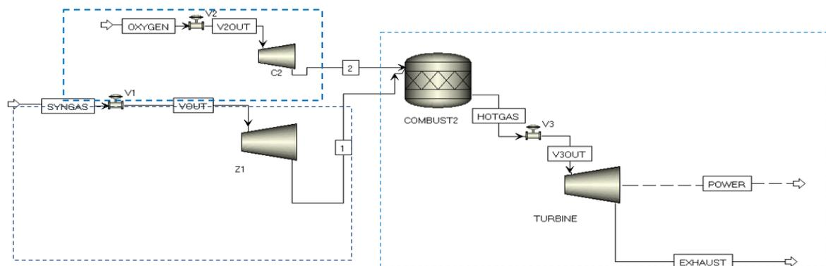
Figure 1: A dynamic BG-CHP flowsheet model in Aspen Plus workspace and model boundaries for NLRAX model
