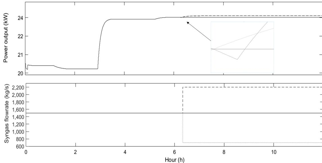
Figure 5: Output responses ( $y_1$ ) due to a  $\pm 700$  point in syngas flowrate (solid line: base case; dash line: positive step change, dotted line: negative step change).
