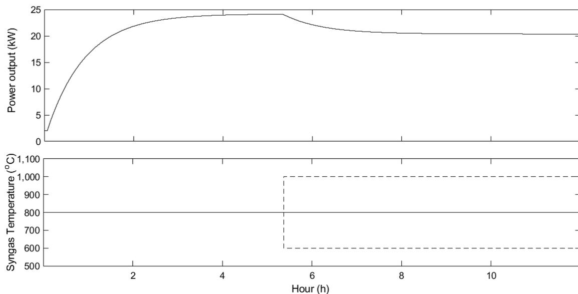
Figure 4: Output responses ( $y_1$ ) due to a  $\pm 200$  point in syngas temperature (solid line: base case; dash line: positive step change and negative step change).
