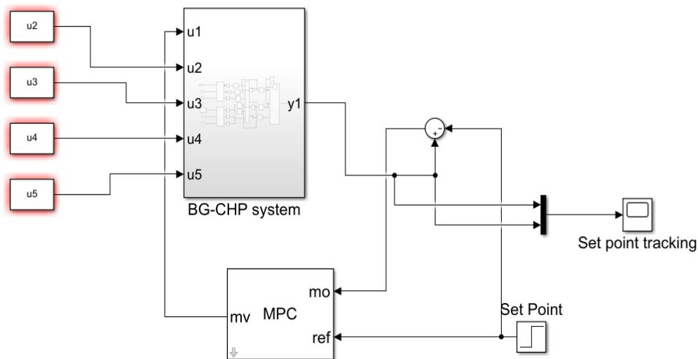
Figure 3: An NLRX-BG-CHP mode embedded with MPC in Simulink/Matlab environment
