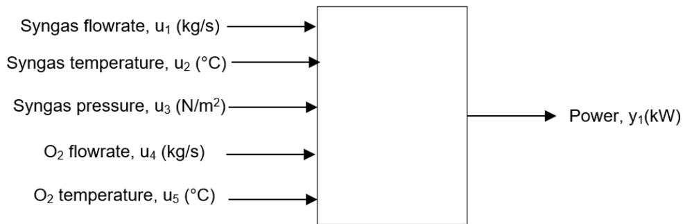
Figure 2: Input-output block diagram for BG-CHP plant
