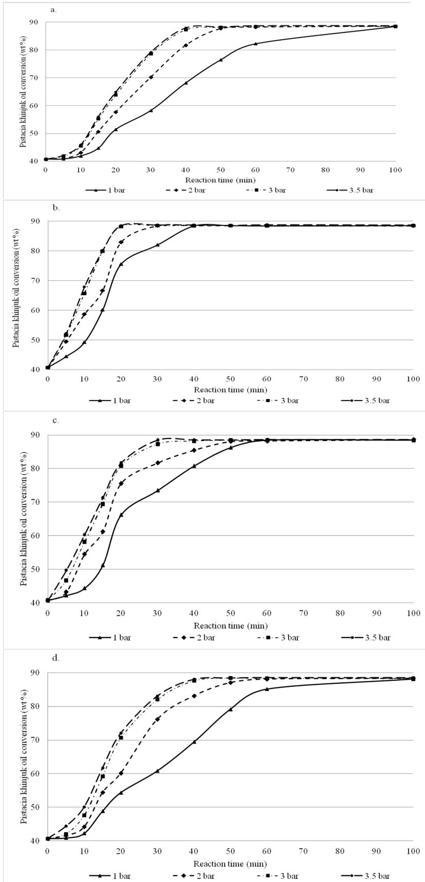
Figure 2: Effect of pressure on methyl ester conversion (a) Plate 1, (b) Plate 2, (c) Plate 3 and (d) Plate 4
