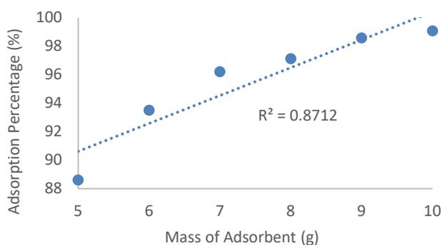
Figure 6: Adsorption percentage vs adsorbent mass
