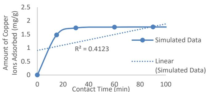
Figure 3: Copper ion adsorbed vs contact time
