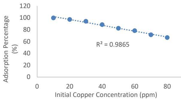
Figure 4: Adsorption percentage vs initial concentration
