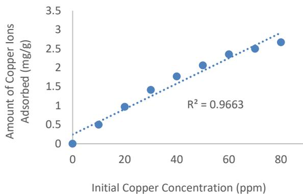
Figure 5: Copper ion adsorbed vs initial concentration
