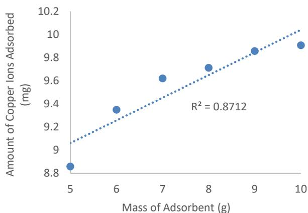
Figure 7: Copper ion adsorbed vs adsorbent mass
