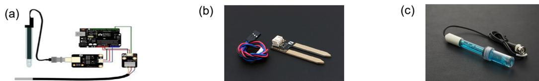
Figure 3: (a) EC meter, (b) Soil moisture sensor, (c) pH sensor
