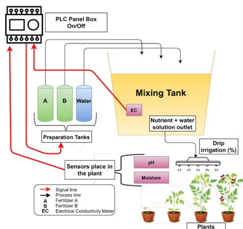
Figure 4: The process diagram of automated blending system in fertigation
