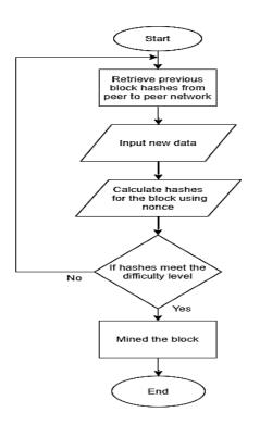
Figure 2 : Flowchart of the mining process.
