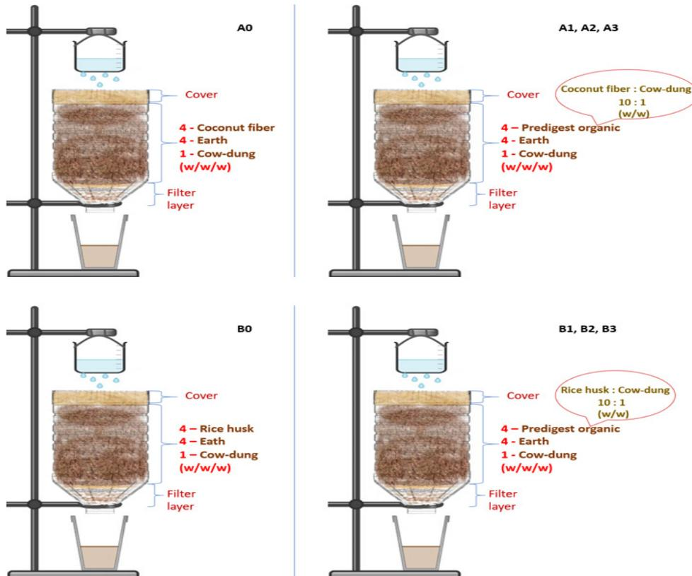
Figure 2: Experimental setup: (A0) control of coconut fiber; (A1, A2, A3) coconut fiber; (B0) control of rice husk; and (B1, B2, B3) rice husk.
