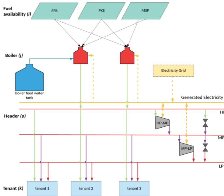
Figure 1: The superstructure of palm oil mill biomass cogeneration system
