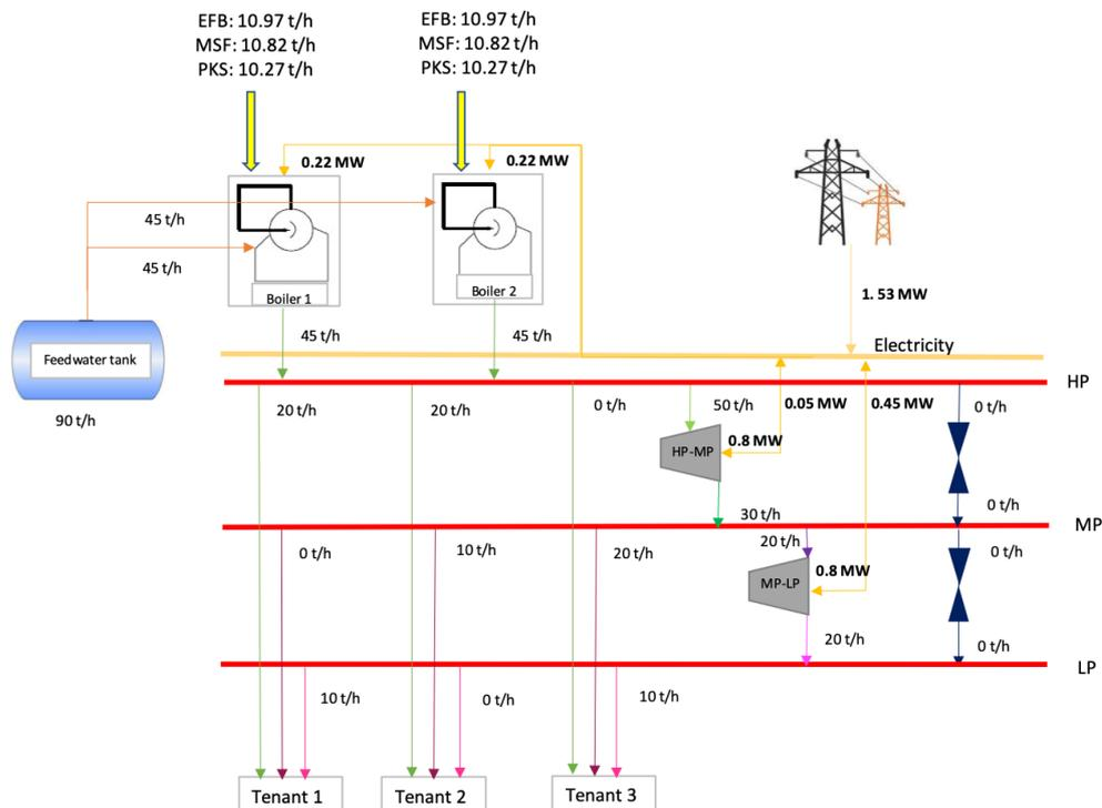
Figure 2: The optimal palm oil mill biomass cogeneration system
