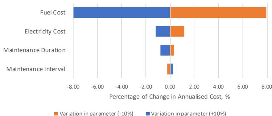
Figure 3: Sensitivity analysis of annualised cost of palm oil mill biomass cogeneration system.
