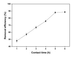
Figure 5: The removal Cr (VI) in metal plating industry wastewater by FAZ
