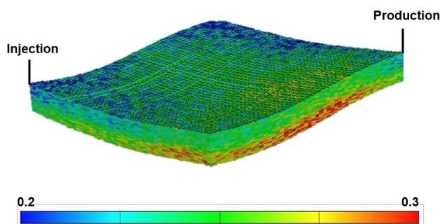
Figure 1: 3D model of porosity
