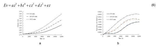
Figure 4: Distance rate at various power supply (a) and evaporation rate at various power supply (b)
