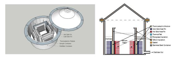
Figure 1: A schematic diagram of a simple integrated distillation vessel using thermoelectric modules
