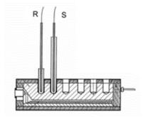
Figure 2: Scheme of the Lütolf-Test according to VDI 2263-1 (1990), with reference and sample vial
