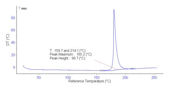
Figure 3: Thermogram of a Lütolf-Test with a sample in which the temperature difference DT is plotted against the reference temperature
