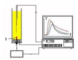
Figure 1: Scheme of the Deflagration test according to VDI 2263-1 (1990), in a 200 ml glass tube with a glow plug (1) as ignition source and temperature recording at 3 levels: low (red), medium (green) and high (blue)
