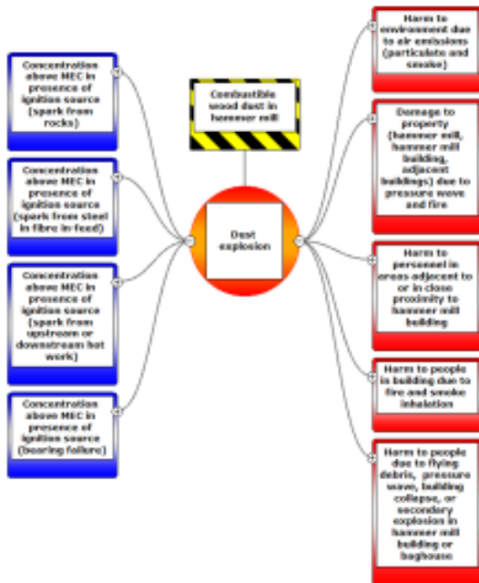
Figure 3: Excerpt of threats and consequences in bowtie for combustibility wood dust in a hammer mill
