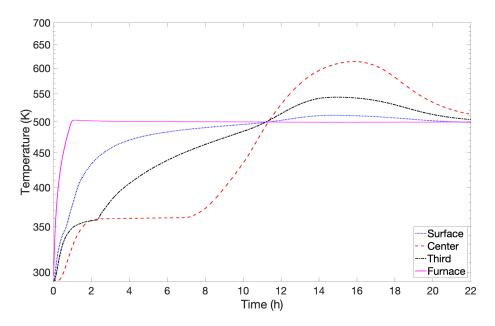
Figure 2: Example of a self-heating test on a soil polluted by hydrocarbons in a 8000 cm3 basket at 230 °C
