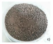
Figure 1: a) Non-passing fraction of the 5 mm sieve, b) sieved hydrocarbons polluted soil, c) depolluted soil
