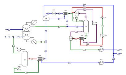
Figure 3: Ethyl acetate production via reactive distillation with separation unit and an MVRHP adapted from (Šulgan, 2021)
