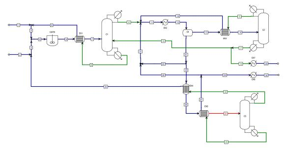
Figure 1: Ethyl acetate production via conventional process set-up adapted from (Šulgan, 2020)
