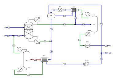
Figure 2: Ethyl acetate production via reactive distillation with a separation unit adapted from (Šulgan, 2020)
