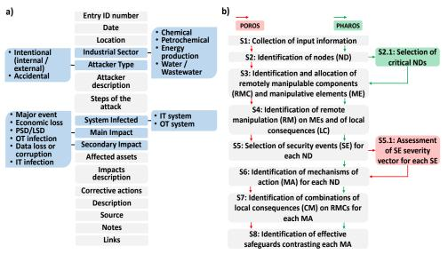
*Figure 1: a)* Structure of the developed database (grey boxes: free text fields; light blue boxes: itemized fields); *b)* Flowchart of POROS (red arrows) and PHAROS (green arrows)
