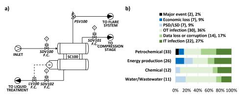
Figure 3: a) Process Flow Diagram (PFD) of the SUC; b) (results from PIA) Share of the impacts of the CSIs recorded vs the industrial sectors
