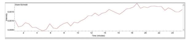
Figure 1: Time dependence of gas release during PLA filament heating at 220 °C
