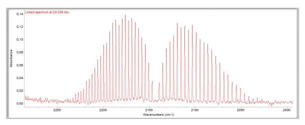
Figure 2: PLA filament spectrum of carbon monoxide, 22nd minute
