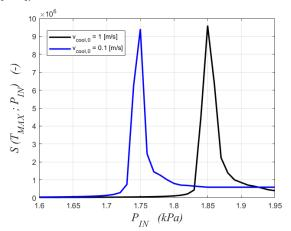
Figure 3: Effect of the jacket fluid velocity on system sensitivity
