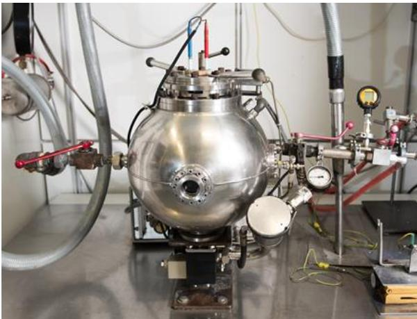
Figure 2: Photo of the explosion sphere
