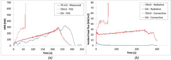
Figure 4: (a) Comparison of measured and predicted HRR for the 0.3 x 0.3m pool fires in the 70  $m^3$  airtight setup and in open atmosphere (OA); (b) Simulated incident heat flux on the pool surface
