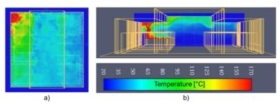
Figure 3: Temperature field at the alarm times in the vertical (a) and cross at the height of the detection system (b) sections.
