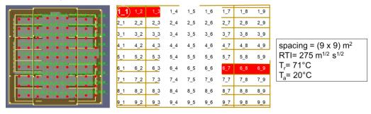
Figure 2: Positioning, nomenclature, and main parameters of the heat detectors employed.
