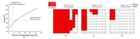
Figure 4: a)  $t_{alarm}$  as a function of the minimum ceiling height ( $h_{min}$ ). Sensors activated in a time of 400 s in the case of TEST1 (b), TEST1 with a  $2h_{min}$  (c) and TEST1 with a  $3h_{min}$  (d).
