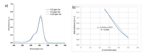
Figure 2: a) Spectra of Rhodamine solutions with different As concentrations and b) Calibration curve ( $\lambda = 553$  nm) for Rhodamine B method
