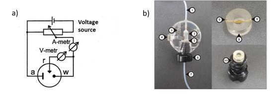
Figure 3: a) electrochemical cell arrangement (a-auxiliary electrode, r-reference electrode, w-working electrode) b) Measuring cell and electrode. 1 Drain, 2 Reference electrode, 3 Auxiliary electrode, 4 Reference solution, 5-8 Measuring electrode, 6-10 sealing screw, 7 Sample load, 9 Gold contacts.
