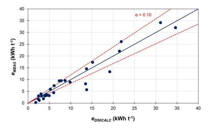
Figure 6: The prediction model of energy demand for knife milling of wheat straw with the confidence belts.
