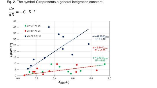
Figure 2: Modelling energy demand on particle size characteristic D<sub>50</sub> and moisture M by Kick theory.
