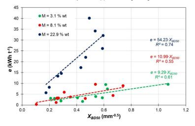
Figure 3: Modelling energy demand on particle size characteristic D<sub>50</sub> and moisture M by Bond theory.
