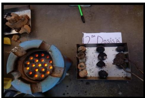
Figure 2: Test of boiling temperature versus burning time of spheres with 500 ml of water
