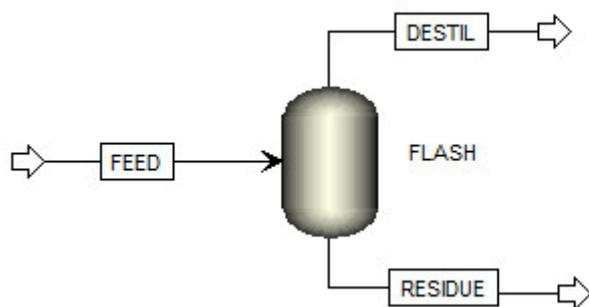
Figure 1: Molecular distillation emulation in the commercial software Aspen Plus®.
