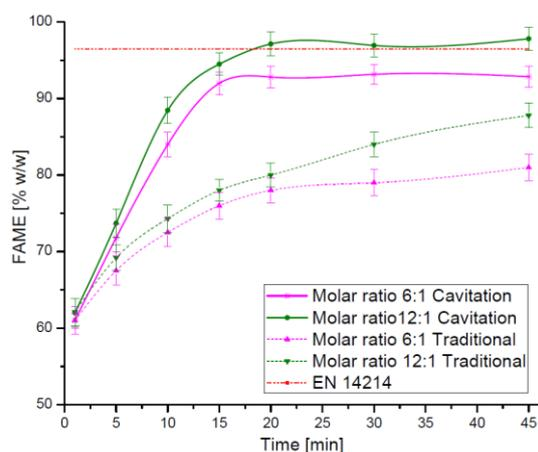
Figure 3: Reaction speed of four experiment.
