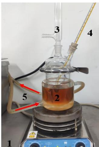
Figure 1: Scheme of the test facility of traditional process (1. Magnetic plate stirrer, 2. Reactor, 3. Condenser, 4. Thermometer, 5. Inlet and outlet of water hot).
