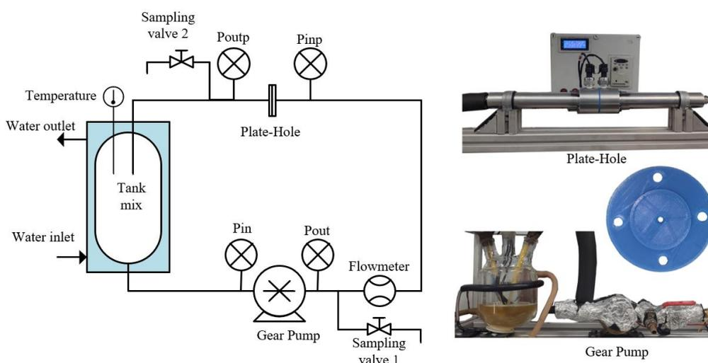
Figure 2: Scheme of the test facility of cavitation hydrodynamics process ( $P_{in}$ : Pressure of inlet in gear pump,  $P_{out}$ : Pressure of outlet in gear pump,  $P_{inp}$ : Pressure of inlet in plate hole,  $P_{outp}$ : Pressure of outlet in plate hole).
