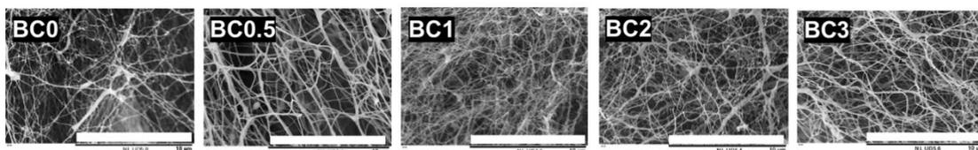
Figure 2: SEM images of freeze-dried BC samples at the magnification of 10000 $\times$ . Scale bars represent 10  $\mu\text{m}$
