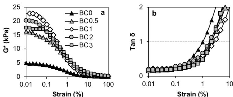
Figure 3: Complex shear modulus (a) and tangent phase angle (b) of hydrogel-like BC pellicles
