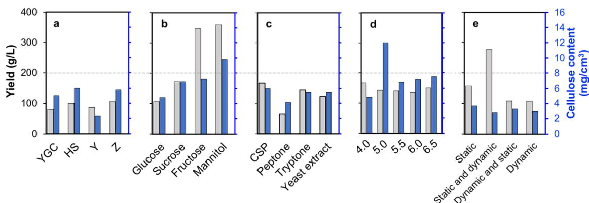
Figure 1: Yield of hydrogel-like BC pellicle (grey bar) and nanocellulose content in the pellicle (blue bar) after cultivating *G. xylinus* in different cell media (a), carbon sources (b), nitrogen sources (c), initial pH values of the cell media (d), and static/dynamic conditions (e).
