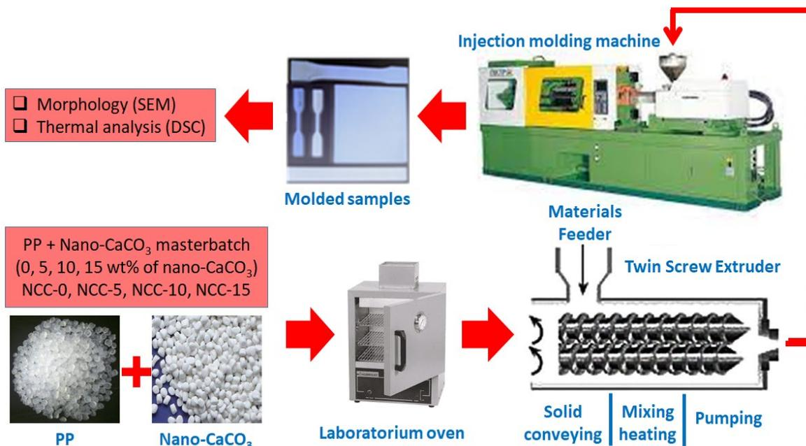
Figure 2: Schematic diagram of PNCCs production
