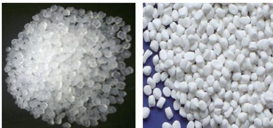
Figure 1: Photographs of polypropylene (PP) pellets (left) and nano-CaCO<sub>3</sub> masterbatch (right)
