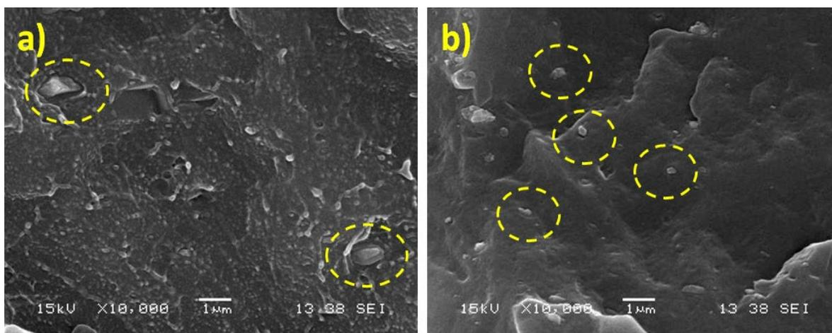
Figure 3: SEM images of a) NCC-5-I and b) NCC-5-II at magnification of 10,000X
