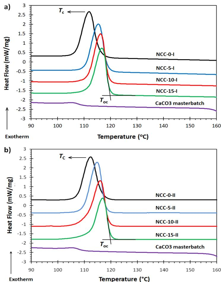
Figure 4: DSC crystallization thermograms of the PNCCs for a) 1<sup>st</sup> cycle and b) 2<sup>nd</sup> cycle
