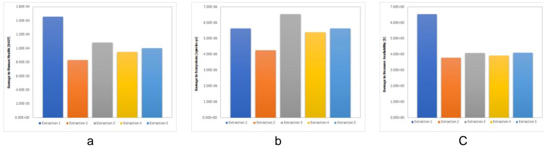
Figure 6: Comparison Results - Endpoint impact categories of the examined extraction process systems (per Kg extract). a. Damage to human health [DALY], b. Damage to ecosystems [species·yr], c. Damage to resource availability [\$].
