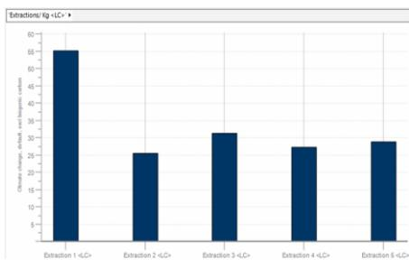
Figure 5: Climate Change, excl biogenic carbon [kg CO<sub>2</sub> eq.] of the examined extraction process systems (per Kg extract).
