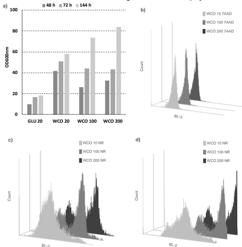
Figure 3: Batch cultivation system *Y. lipolytica* W29 in rich medium with Glucose 20 g/L, WCO 20, 100 and 200 g/L: a) cell growth profiles (OD<sub>600</sub>) at three time intervals (48, 72 and 144 h); b) 7-AAD fluorescence intensity (BL-3); c) NR fluorescence intensity (BL-3); d) NR fluorescence intensity (BL-2). Fluorescence intensities for each dye were determined at 144 h in rich medium with WCO 20, 100 and 200 g/L.
