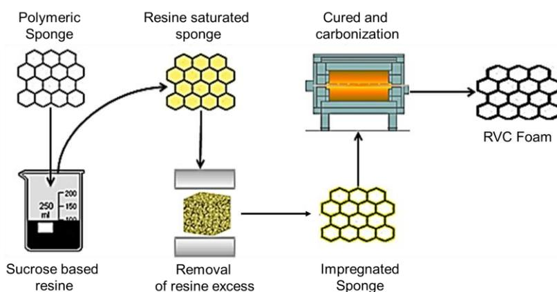
Figure 1. Fabrication process of reticulated vitreous carbon foams by template method.
