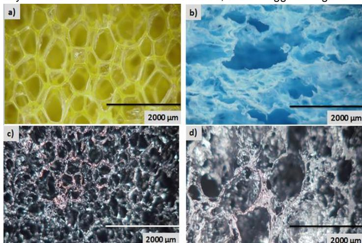
Figure 3: Confocal micrographics of a) polyurethane, b) cellulose sponges and RVC foams elaborated with c) polyurethane and d) cellulose as sacrificial templates.
