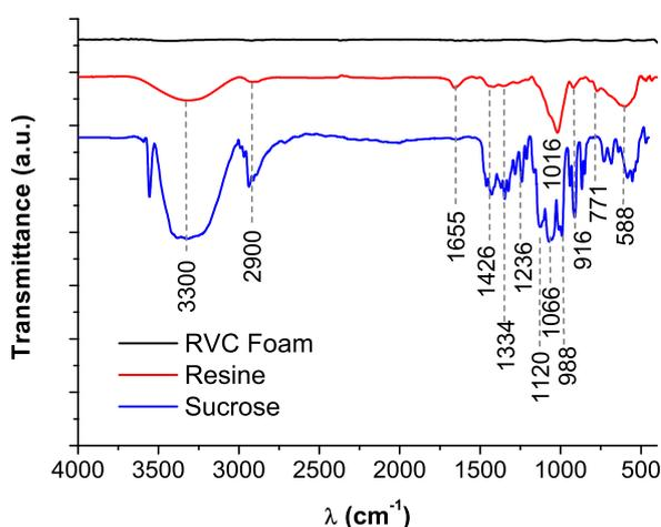
Figure 2: FTIR spectrum for sucrose, resin and RVC foam
