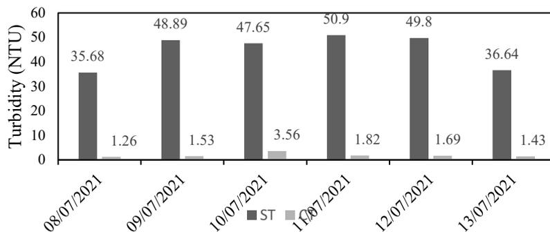
Figure 3: Results of turbidity measurements in the installation of the filter in the pilot plant of the runoff water of the San Lorenzo de Moyobamba sector - NTU (ST: Without treatment, CT: with treatment)
