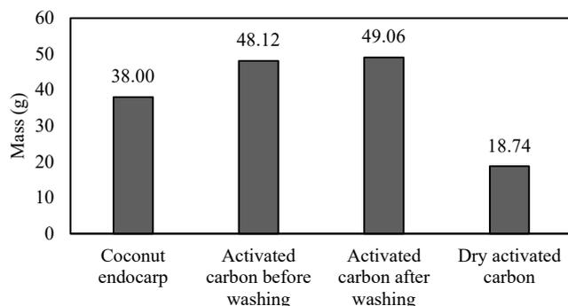
Figure 1: Average weight of activated carbon in the stages of the carbonization process (grams)
