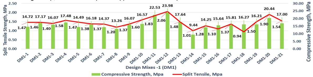
Figure 3: Design Mixes – 1 (DM1) Compressive and Split Tensile Strength Test Results
