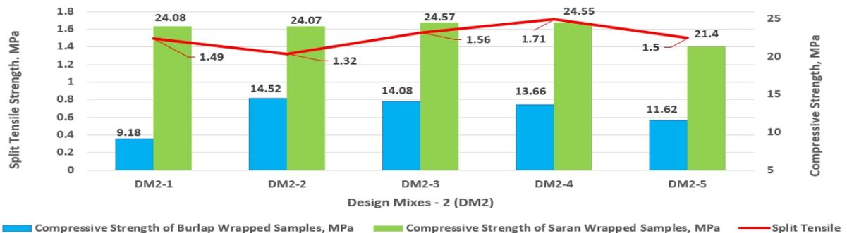
Figure 4: Correlation of Compressive and Split Tensile Strength
