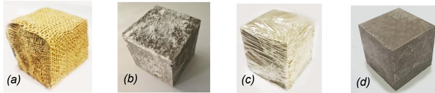
Figure 2: Geopolymer Mortar Efflorescence: (a) Geopolymer wrapped with burlap; (b) Occurrence of efflorescence; (c) Geopolymer with saran wrap; (d) Non-occurrence of efflorescence
