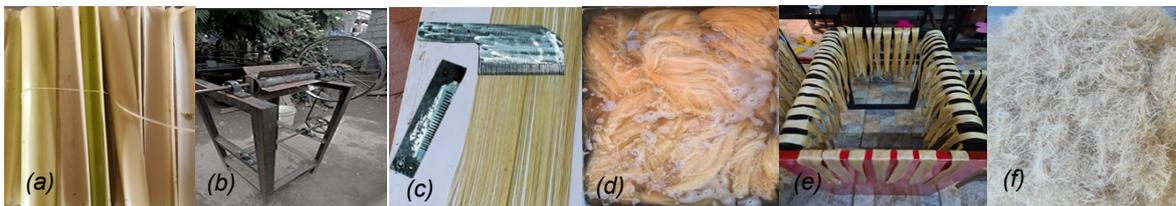
Figure 1: BF Extraction and Treatment Flow (a) Banana pseudostem, (b) decorticator (c) BF stripping tool (d) NaOH Treatment (e) Drying of treated BFs (f) 1cm short BFs
