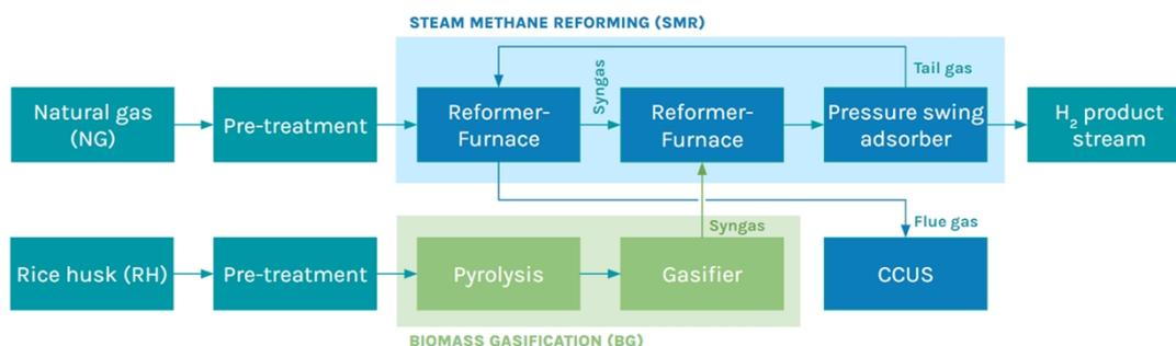
Figure 1: Block-flow diagram of proposed novel teal hydrogen production plant
