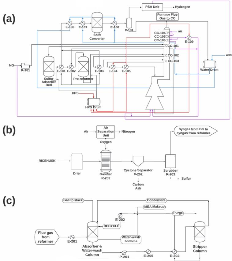
Figure 2: Process flow diagrams of the proposed teal  $H_2$  plant, (a) steam-methane reforming facility and its utilities, (b) biomass gasification, and (c) carbon capture. The blue lines represent the cold utility stream, the red lines represent the hot utility stream, and the purple lines represent the furnace feed
