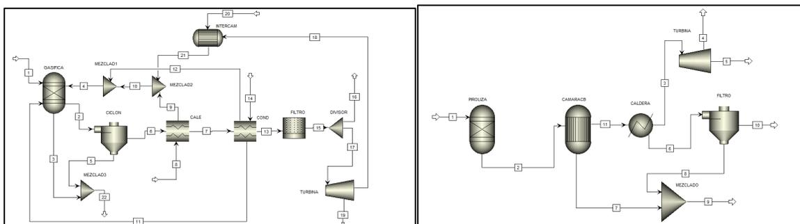
Figure 4: Left: Gasification process flow diagram using Aspen Plus V8.8 software, implementing the POLYNRTL method. Right: Flow diagram of the pyrolysis process using Aspen Plus V8.8 software, implementing the POLYNRTL method.
