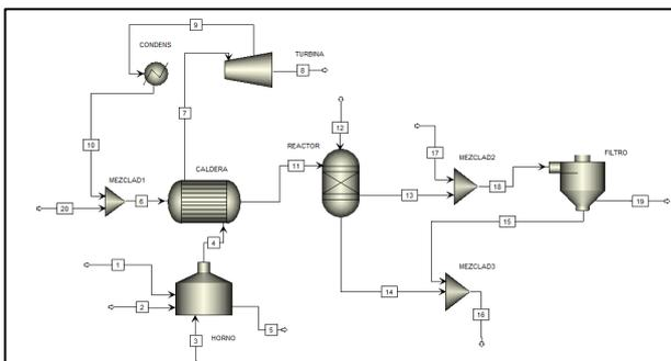
Figure 3: Flow diagram of the incineration process using Aspen Plus V8.8 software, implementing the POLYNRTL method.
