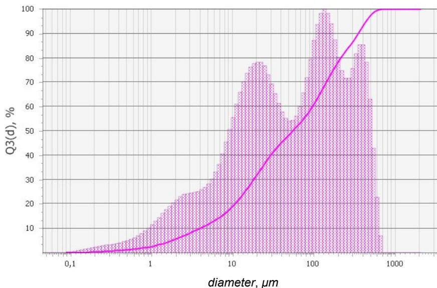
Figure 2: Granulometric composition of technogenic basalt powder
