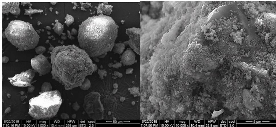
Figure 3: Microstructure of technogenic basalt powder
