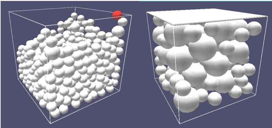
Figure 1: Model of random packing of particles in the system gypsum binder-technogenic basalt powder
