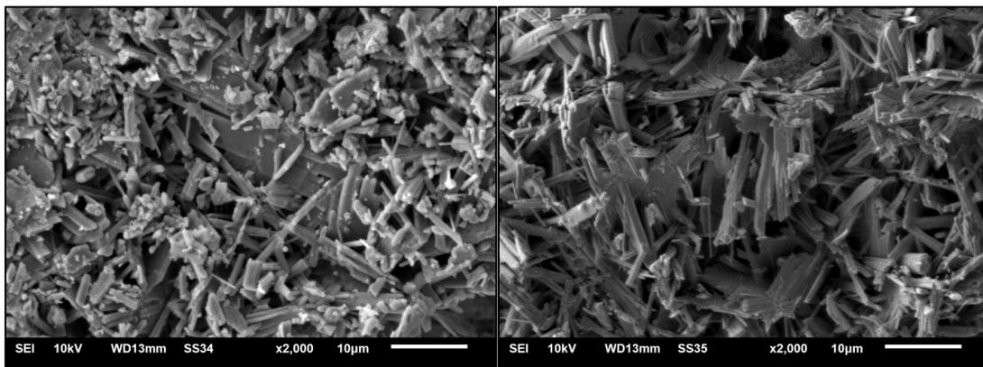
Figure 5: Microstructure of pure gypsum binder (right) and modified with technogenic basalt powder (left)
