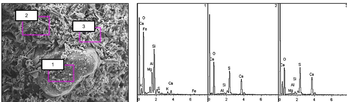
Figure 6: Microstructure of gypsum stone modified with technogenic basalt powder, aluminosilicate ash component and slaked lime and obtained spectra
