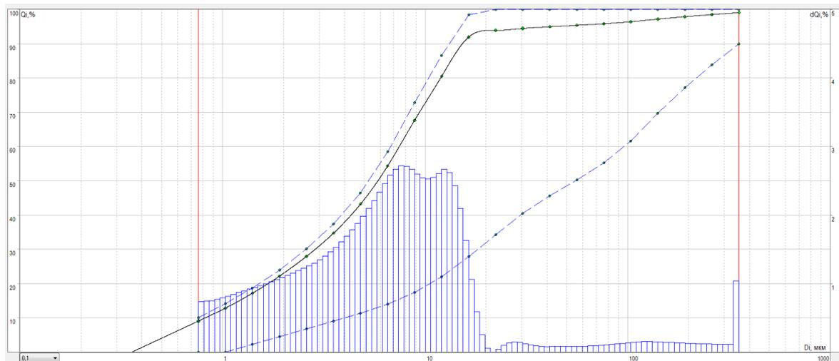
Figure 4: Differential and integral distribution in the composition of a mixture of gypsum binder and ground technogenic basalt powder
