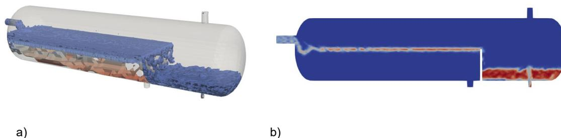
Figure 8: 3D Model of the 3-phase separator (a) and vertical slice displaying oil layer in the separator (b)
