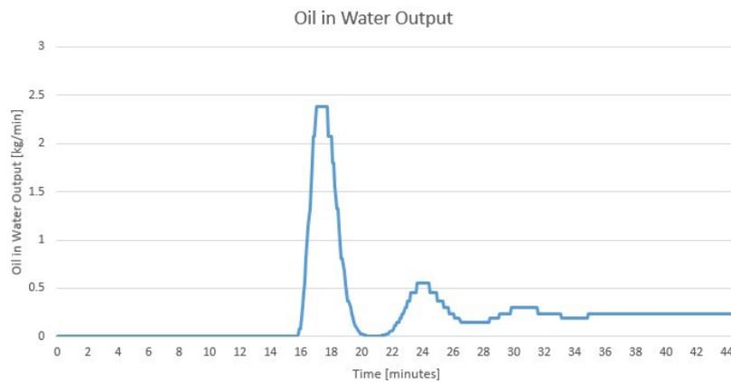
Figure 5: Dynamic state of oil residuals in water output at start-up
