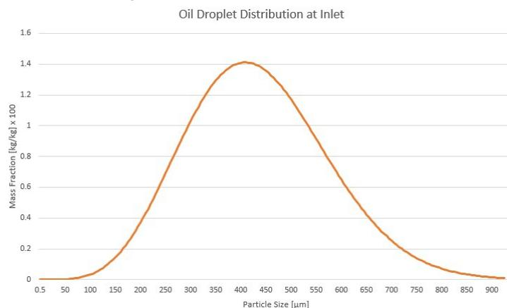
Figure 3: Initial starting point for oil droplet distribution in the water phase at the inlet
