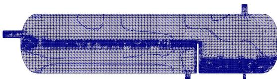
Figure 6: Adaptive mesh refinement at the phase boundaries of oil, water and gas
