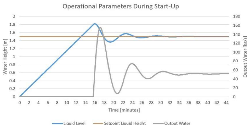
Figure 4: Dynamic states of the operational parameters of a 3-phase separator at start-up
