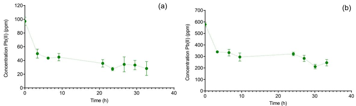
Figure 4: (a) Pb(II) removal for B80 samples and (b) Pb(II) removal for B500 samples
