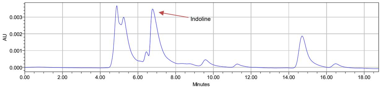
Figure 3: B80 sample HPLC spectra with the final method
