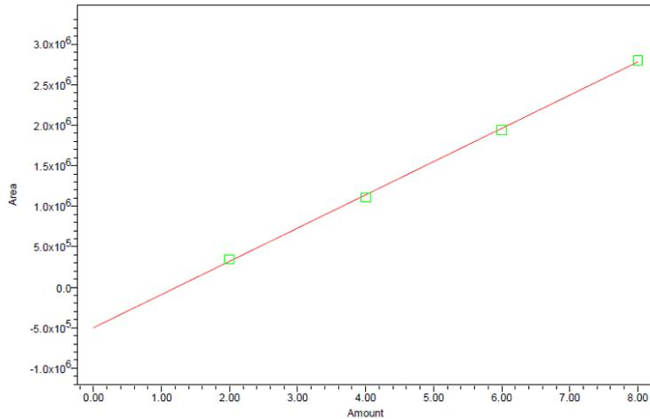
Figure 2: Calibration results for Indoline
