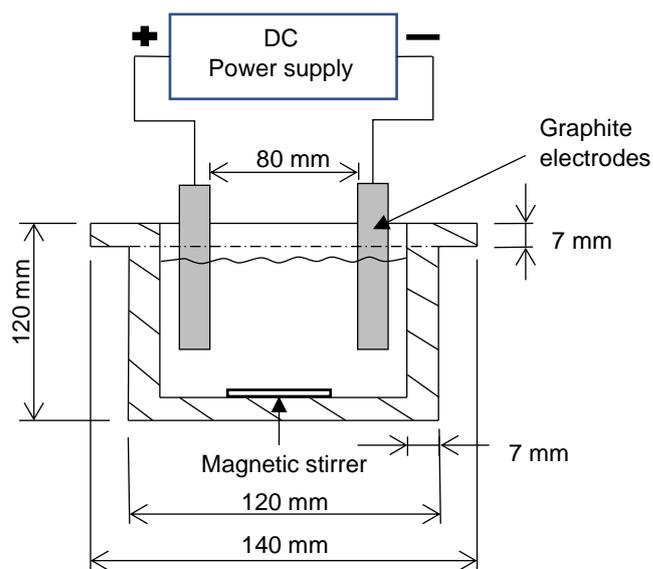
Figure 1: Schematic view of the electrochemical reactor
